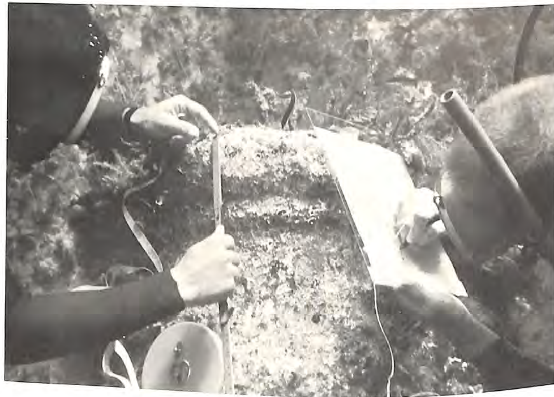
As Nikos Kartelias measures the astragal of a column, Roger Wallihan records the data on a sheet of plastic which is taped to a plexiglass "board."
