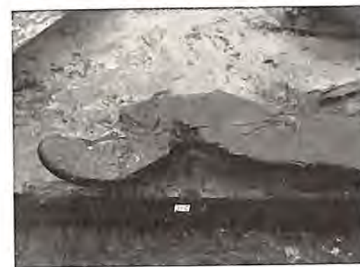
Figure 14. Section 3, GXB. Frame cut to fit over the deckline wale.
