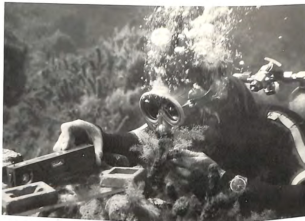
Using sights mounted on a weighted spirit level, a member of the expedition takes a bearing on a surveying rod held by another diver in the wreck (outside the picture).
