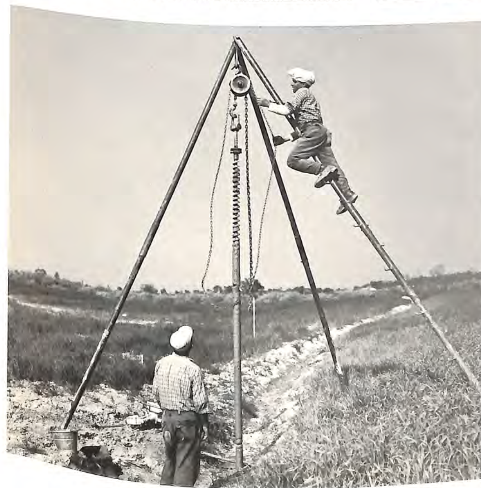
(Upper left) The McCullough drill being used by Domenico Falcone and Giuseppe Dattoli. (Left) Auger-bit of the McCullough drill being pulled out with its sample by a chain-hoist and tripod. (Above) Extracting the finds from the mud on the auger-bit and laying them out on a board in the order of their stratification. Left to right: Donald Brown, Orio Miggiano, who was the Government representative, and Domenico.
