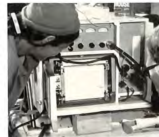
Figure 7. The magnetometer chart on the ship's deck showing an anomaly picked up by the detector in the water.
